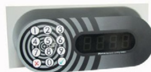
Display Combo: 4 digit LED display and a combination of keypad to enter PIN code and RFID reader.
