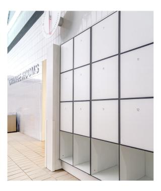
Each locker door was designed clean lined – no handles or individual RFID readers on the front of the doors.
